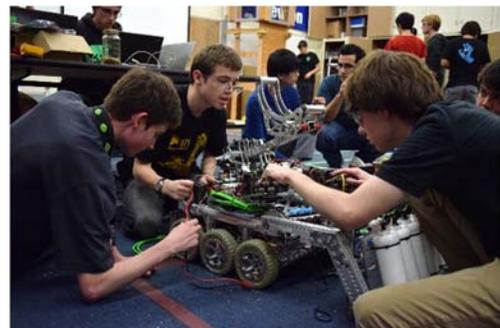
by 19 inches, and will debut at Madtown Throwdown. It contains a turret, catapult, and a smaller drive base. The turret has 180°-degree rotation capability, and carries the catapult on the top. The catapult is designed to have an adjustable shot, have a stop length, and be able to easily scoop boulders. Another feature is its vision tracking, which allows it to make both high and low goals.
