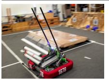
Introducing our competition robot for this season, Tangerine Tumbler! With a frame of 26 by 26 inches, Tangerine Tumbler weighs about 90 pounds. It has a rotatable elevator with an intake made of silicone rollers to grab cubes and cones. The 43-inch long forks are rods of carbon fiber that allow us to quickly do a buddy climb during endgame. The current packaging of the robot allows
