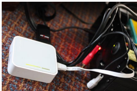
Figure 2 3G dongle, router, and part of the case
